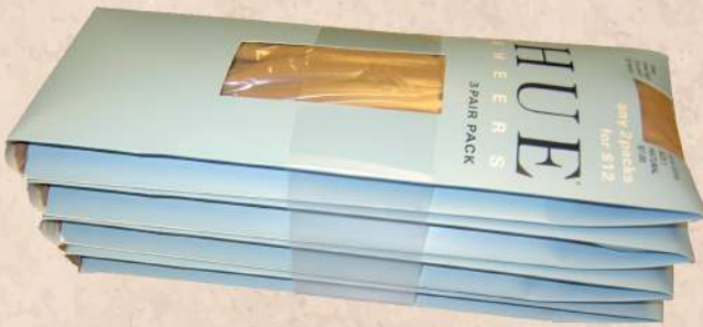
BUNDLING PRODUCT USING ULTRASONIC BANDING
