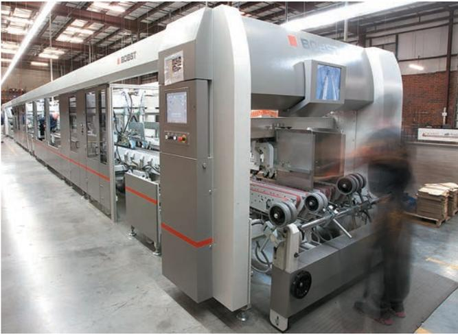
Multi-directional folding and gluing for heavier board is achieved, thanks to the Gyrobox module, below, on the Bobst MASTERFOLD.
