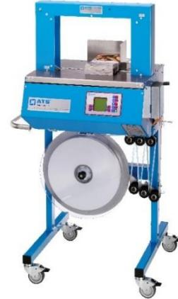
be used as a stand alone unit or ordered with special options for integration into a production line. *This machine utilizes a wide range of materials including white paper, brown paper and clear films along with custom printed materials for branding and the ability to print on-demand.*
